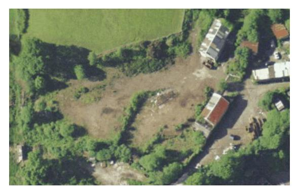
Planning consent was granted subject to several conditions requiring the developer to investigate the land for contamination and identify a remediation strategy to reduce any risks to an acceptable level. The site was investigated and found to be contaminated with petroleum/diesel range hydrocarbons, asbestos fibres and heavy metals.
